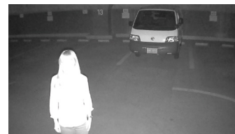
Conventional IR technology (cannot identify close objects due to overexposure)
