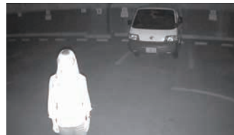
Without Advanced IR mode (cannot identify close objects due to overexposure)
