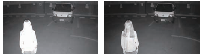
Without Advanced IR mode (cannot identify close objects due to overexposure)
